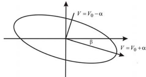
Figure 1 Ellipse of PS wave velocity which indicates the azimuthal variation of PS wave velocity in azimuthal anisotropic media.
