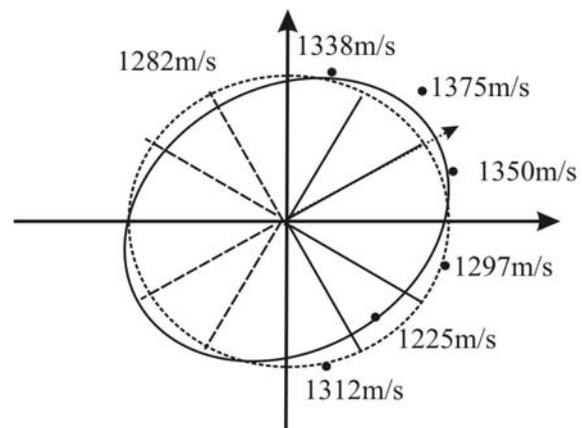
Figure 5. Example of measured PS wave velocity and ellipse fitting results.
