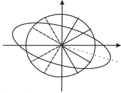
Figure 2. Seismic data is separated into sections according to azimuth. As the data is symmetrical with azimuth, all data section are combined into section between  $0^\circ$  and  $180^\circ$ .
