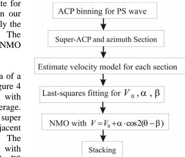
Figure 3. Processing flow for compensating
