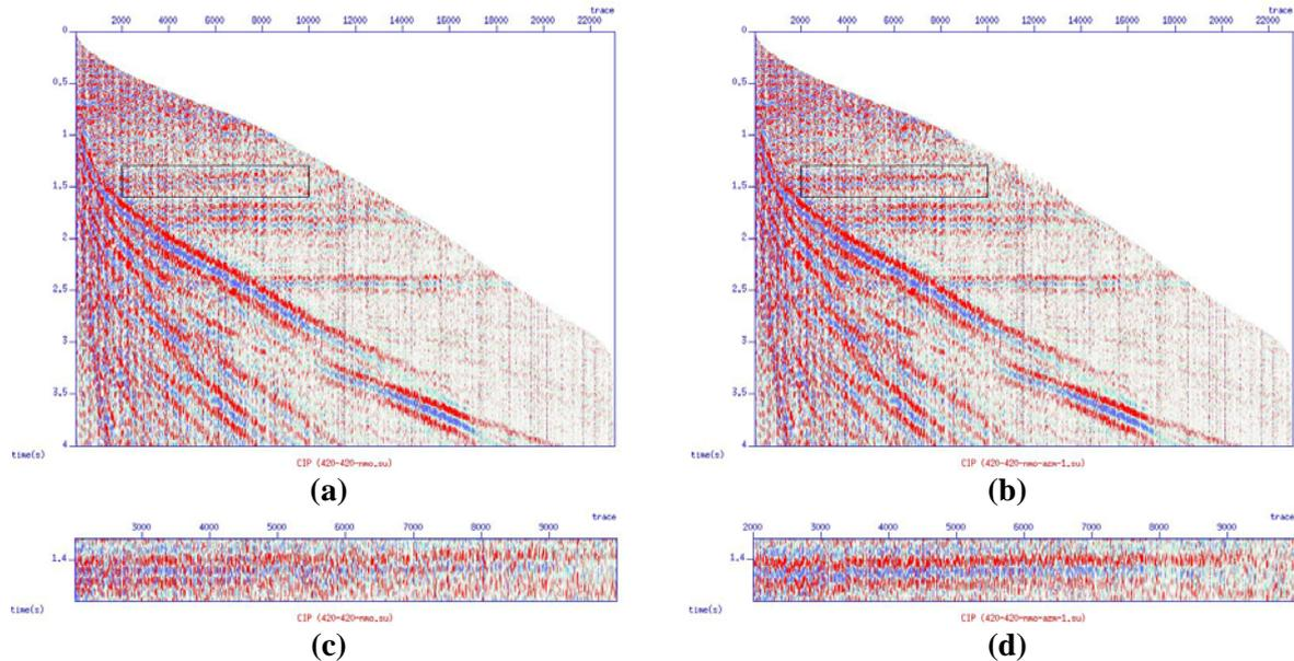
Figure 6. (a) Residual NMO without azimuthal variation velocity in a super ACP gather. (b) Residual NMO with azimuthal variation velocity in the same ACP super-gather. (c) and (d) are enlarged picture of the rectangle in (a) and (b), respectively, and indicate the event which we measured its azimuthal anisotropy and applied the velocity with and without azimuthal variation.
