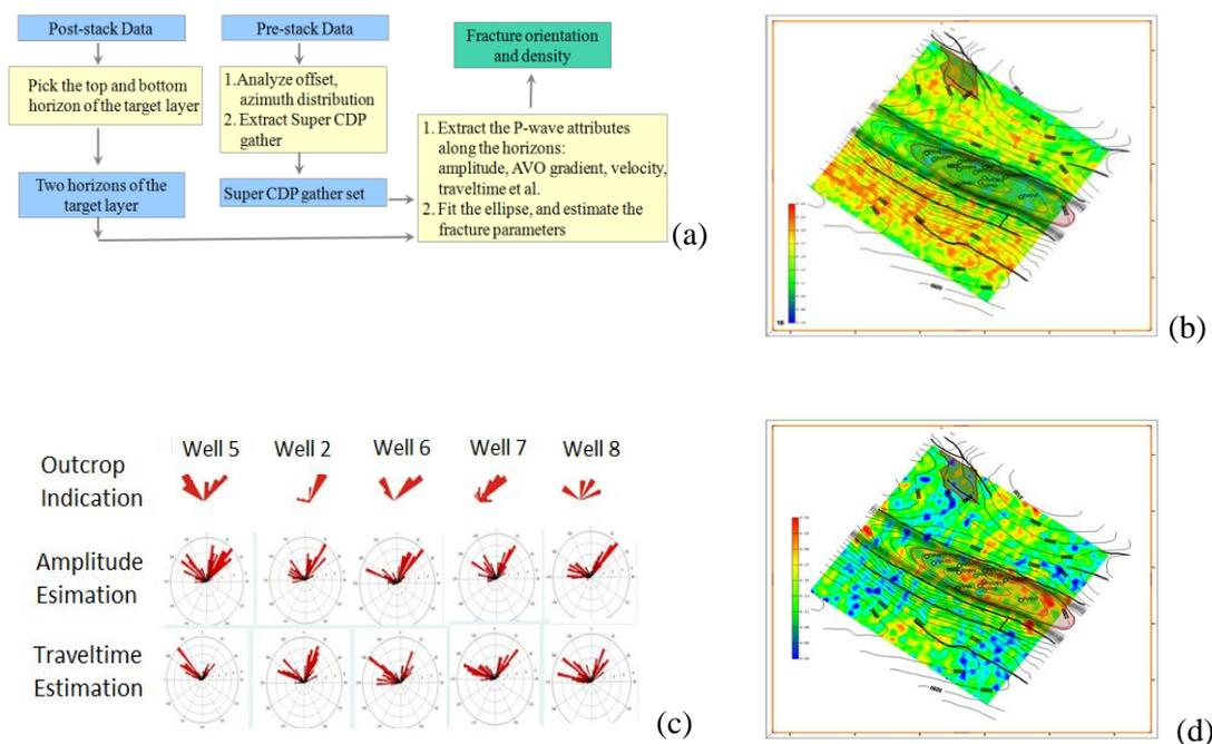
**Figure 4.** (a) workflow for fracture estimation; (b) fracture density prediction using traveltimes attributes overlaid with the contour of the reservoir; (c) comparison of fracture orientation at the well locations obtained using different methods: outcrop and log analysis, prestack amplitude analysis and prestack traveltimes analysis; (d) fracture density prediction using prestack amplitude attributes overlaid with the contour of the reservoir;
