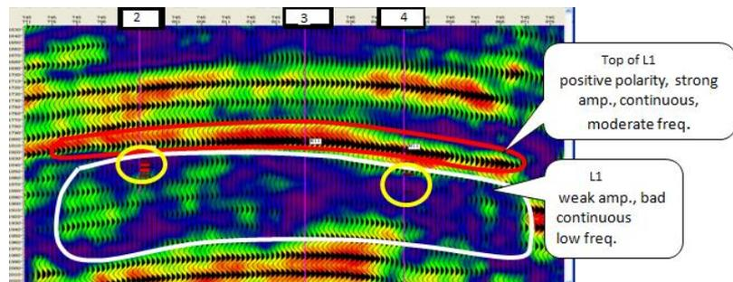
**Figure 3.** Instantaneous frequency map covered with seismic section and three well logs (Well 2, 3 and 4, see Figure 2e),
