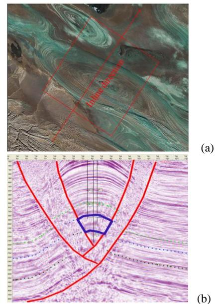
**Figure 1.** (a) Google map view from the space; (b) a seismic section running through the anticline with the anticline in the middle, two reverse fault zones (between the two set of red lines) at the flanks, and the target reservoir just beneath the anticline (in blue closed line).
