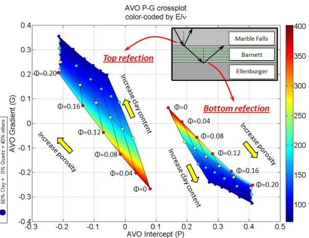
**Figure 7** Seismic AVO intercept-gradient crossplot coloured-code by brittleness index, showing the effect of mineralogical mixtures and porosity.
