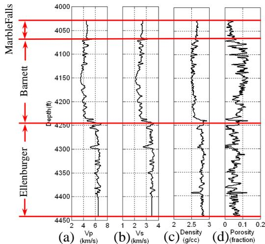
**Figure 6** Well logs for the formations of Marble Falls, Barnett, and Ellenburger, showing (a) P-wave velocity, (b) S-wave velocity, (c) density, and (d) porosity.
