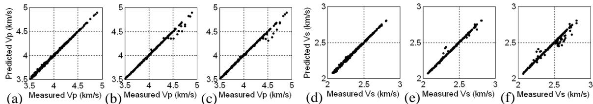
**Figure 3** Cross-plot of the measured  $V_p$  versus the predicted  $V_p$  using (a) single porosity model, (b) traditional dual porosity model, and (c) explicit dual porosity model. (d), (e), and (f) are the corresponding cross-plots of the measured  $V_s$  versus the predicted  $V_s$ .
