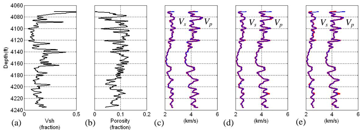
**Figure 2** (a) Shale volume, (b) Total porosity, and Measured (red) and predicted (blue)  $V_p$  and  $V_s$  by fitting modeling data to sonic logs using (c) single porosity model, (d) traditional dual porosity model, and (e) explicit dual porosity mode.
