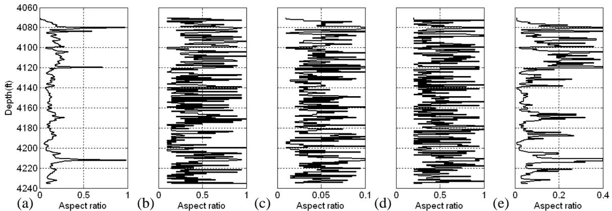
**Figure 4** (a) Aspect ratio derived using the single porosity model. (b) and (c) are aspect ratios of pores associated with non-clay mineral grains and clays derived using the traditional dual porosity. (d) and (e) are those derived using the explicit dual porosity model.
