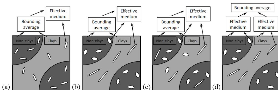
**Figure 1** Schematic representation of different rock physics models for effective medium with (a) single porosity, (b) dual porosity with cracks in clays and stiff pores in minerals of non-clays, (c) dual porosity with complex distributions of cracks and stiff pores in the mixture of clays and non-clays. Figure 1-(d) is our new rock physics model for rock of dual porosity.
