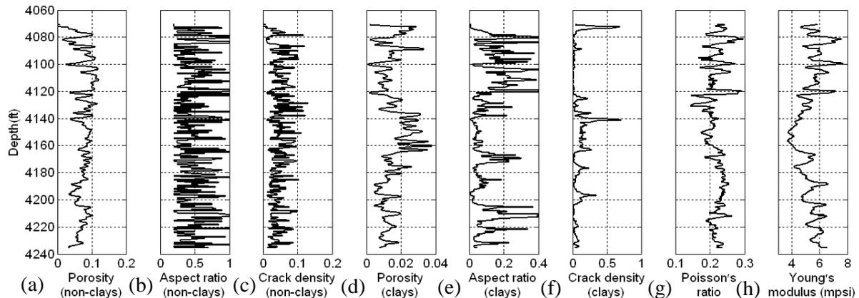
**Figure 6** (a) Porosity, (b) Aspect ratio, and (c) Crack density associated with pores for non-clay minerals. (d), (e), (f) are those for clays. All these aspect ratios are derived using our explicit dual porosity model. (g) and (h) are Poisson's ratio and Young's modulus, respectively.
