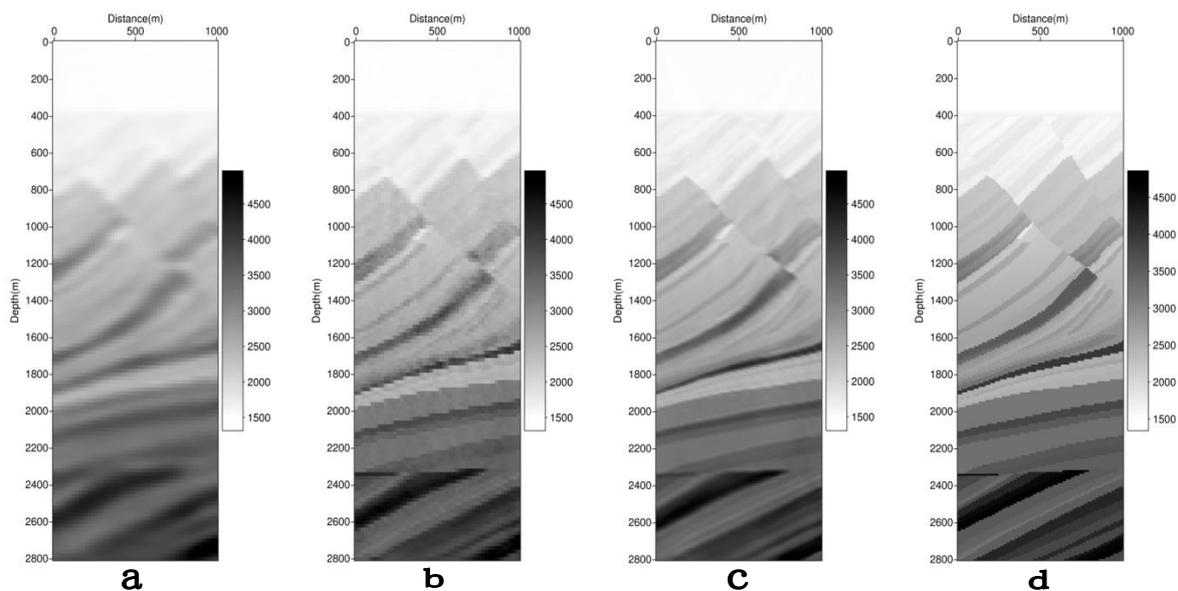
**Figure 3** Multi-scale inversion results on the target zone of the Marmousi model. (a) Inversion result using 20m-spaced grids and 0-20 bandwidth. (b) Inversion result using 20m-spaced grids and 0-50 bandwidth. (c) Inversion result using 10m-spaced grids and 0-50 bandwidth. (d) True velocity model
