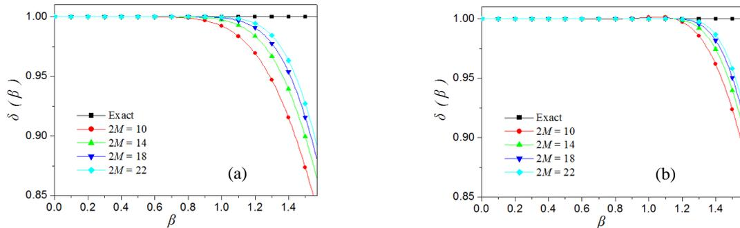
**Figure 1** Plot of numerical dispersion curves by (a) the Taylor-series expansion SFD scheme and (b) the sampling interpolation SFD scheme for different operator lengths.
