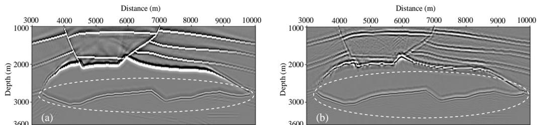
**Figure 5** Elastic RTM result using the sampling interpolation SFD scheme with fixed difference operator lengths for the modified salt model: (a) PP image, (b) PS image.
