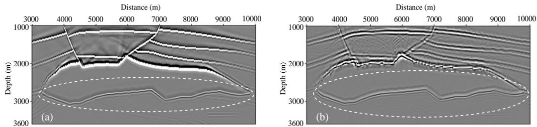
**Figure 6** Elastic RTM result using the sampling interpolation SFD scheme with adaptive variable difference operator lengths for the modified salt model: (a) PP image, (b) PS image.
