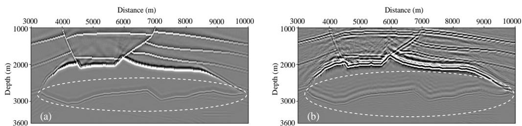
**Figure 4** Elastic RTM result using the Taylor-series expansion SFD scheme with fixed difference operator lengths for the modified salt model: (a) PP image, (b) PS image.
