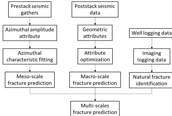
**Figure 1** The procedure for integrated multi-scale fracture prediction with prestack and poststack seismic and well logging.
