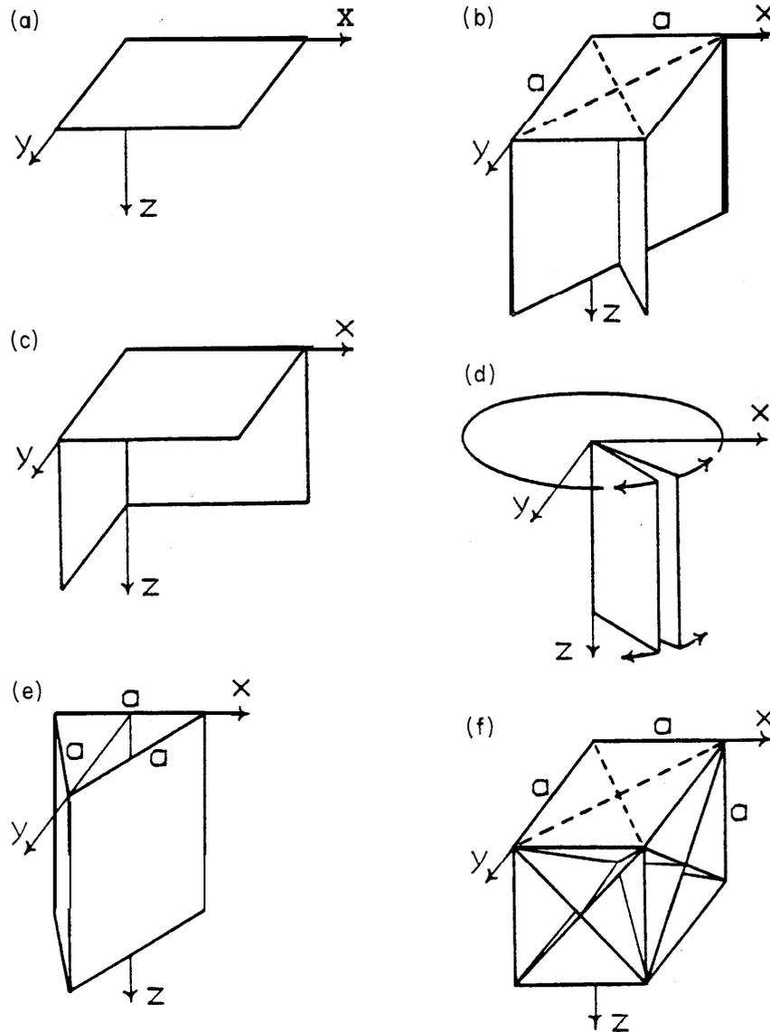
FIG. 3. Spatial orientations of symmetry planes of the more common symmetry systems: (a) monoclinic, (b) tetragonal, (c) orthorhombic, (d) hexagonal, (e) trigonal, and (f) cubic. The triclinic system (Fig. 2) has no symmetry planes, and every plane of an isotropic system is a symmetry plane. (After Crampin 1984a.)
