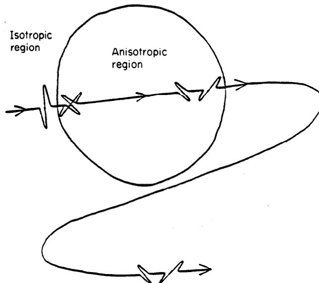
**FIG. 4.** Schematic illustration of shear-wave splitting. The velocities and orientations of the split shear-waves are **fixed** by the particular direction of propagation through the anisotropic symmetry.
