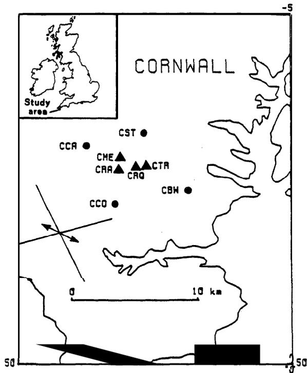
Fig. 1. Map showing locations of the surface network of seismic stations around the Rosemanowes Quarry (CRQ) with three-component stations marked with triangles (after Roberts and Crampin 1986). Arrows mark the directions of maximum compressional stress at the nearby South Crofty mine and lines mark the directions of joints at surface outcrops (Batchelor 1984).
