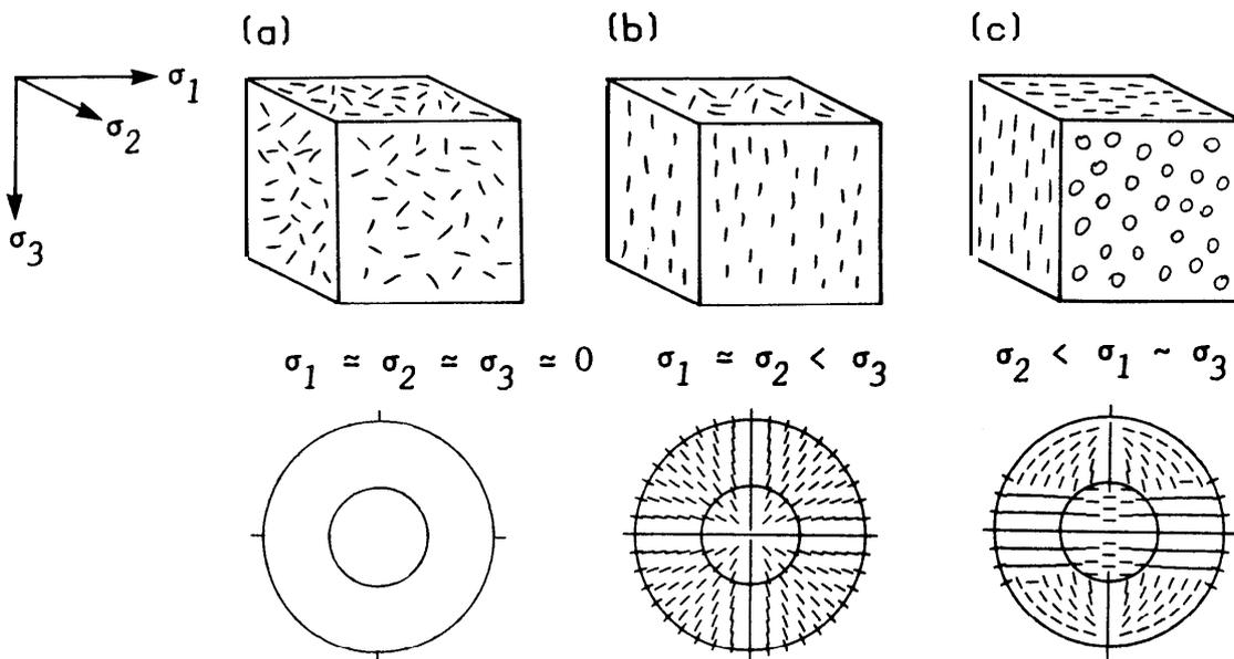
**FIG. 4.** Expected orientations of microcracks in laboratory experiments for a range of stress relationships: (a)  $\sigma_1 \approx \sigma_2 \approx \sigma_3 \approx 0$ ; (b)  $\sigma_1 \approx \sigma_2 < \sigma_3$ ; and (c)  $\sigma_2 < \sigma_1 \sim \sigma_3$ . Notation as in Fig. 2. The blank equal-area projection indicates propagation through randomly oriented cracks where there are no preferred shear-wave polarizations.
