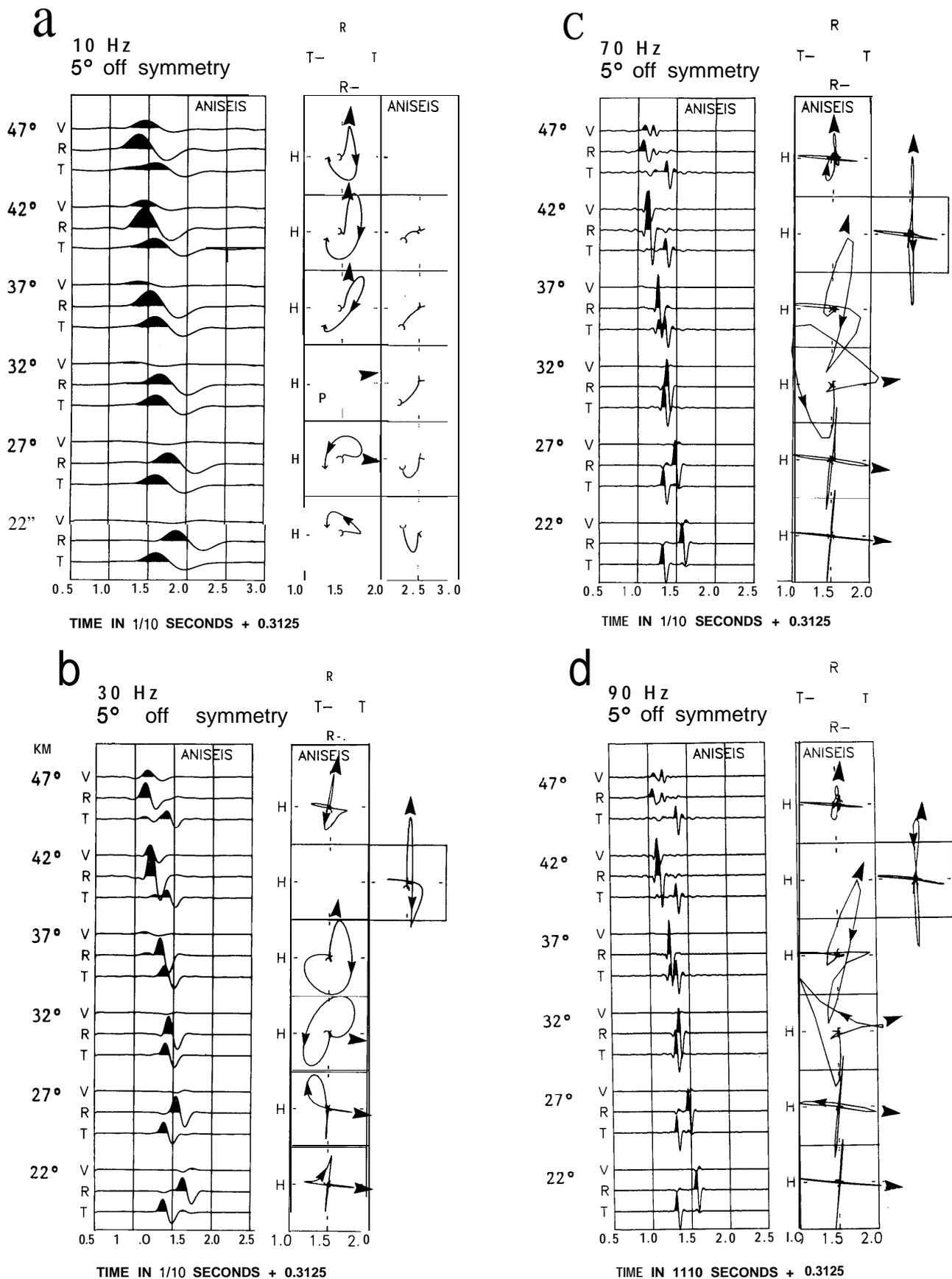
Figure 9. Synthetic seismograms for an *SH45SV* source along the ray paths in the vertical arc  $5^\circ$  from sagittal symmetry [the left line of dots in the insets to Figs 5(b) and (e)], for a source with frequencies: (a) 10 Hz; (b) 30 Hz; (c) 70 Hz; and (d) 90 Hz. Notation as in Fig. 8.
