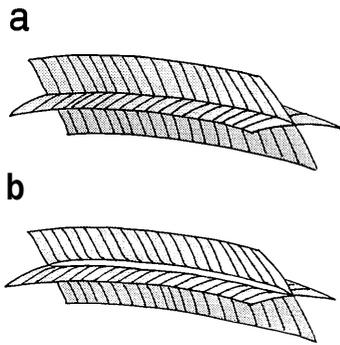
**Figure 2.** Schematic illustration of: (a) a line singularity in hexagonal symmetry, where the two phase-velocity sheets intersect; and (b) the pulling apart of the inner and outer phase-velocity sheets into a ring pinch when there is a small perturbation to the hexagonal symmetry. Note point singularities at both ends of the section illustrated.
