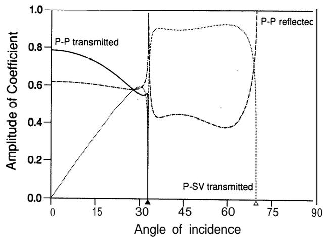
Figure 1. Downgoing plane-wave reflection and transmission coefficients for **P** waves incident from above a water-solid interface. The solid medium has  $\alpha = 2.77 \text{ km s}^{-1}$ ,  $\beta = 1.60 \text{ km s}^{-1}$  and a density of  $2.3 \text{ g cm}^{-3}$ . Solid and open triangles mark the critical angles for **P** waves and **S** waves in the lower medium respectively.
