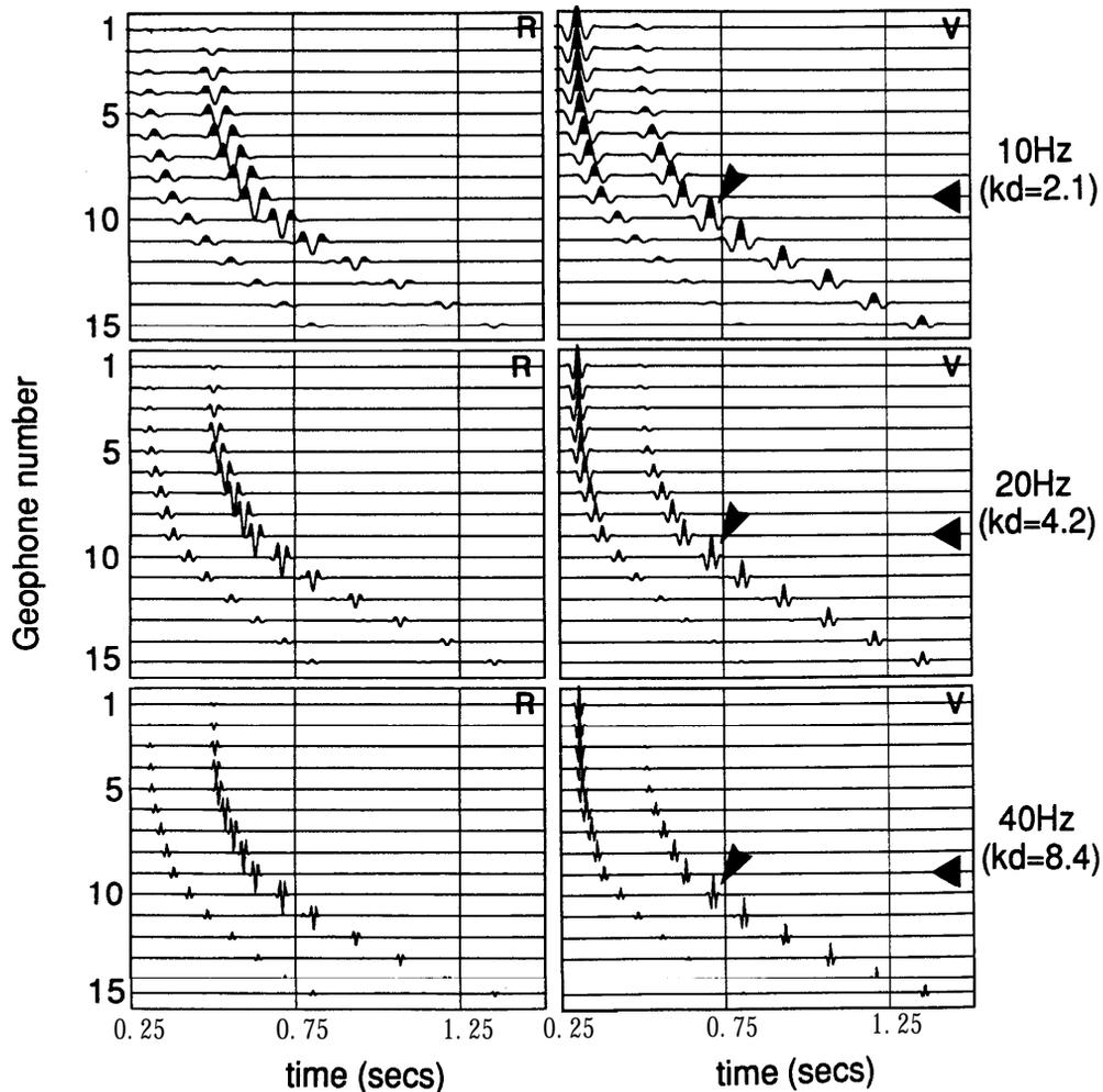
Figure 4. Radial- and vertical-component synthetic seismograms from numerical calculations based on the reflectivity method. The model is identical to that used for Fig. 3, except that the multiples in the water layer have been mathematically suppressed by setting the downgoing P-wave reflection to zero. Notation and normalization as in Fig. 3.
