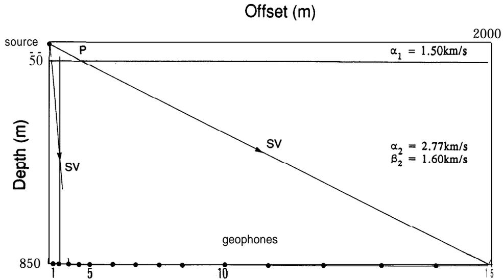
Figure 2. Acquisition geometry used in the numerical modelling to simulate a range of converted wave behaviour. An explosive source is positioned 3 m from the free surface of a water layer 50 m thick. Fifteen geophones are positioned at offsets of 25, 50, 100, 150, 200, 300, 400, 500, 600, 800, 1000, 1250, 1500, 1750 and 2000 m, at a common depth of 850 m.
