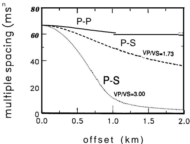
Figure 6. Periodicity of water-column multiples for direct **P** wave (solid line) and converted **SV**-wave arrivals (dashed line for  $V_P/V_S$  of 1.73 and dotted line for  $V_P/V_S$  of 3.0).
