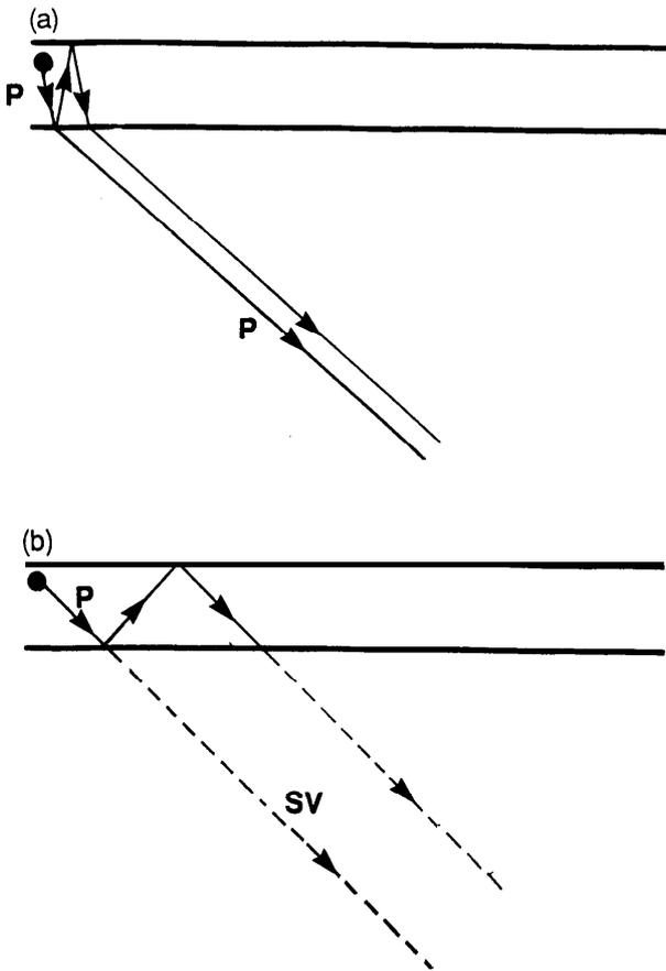
Figure 5. Illustration of different ray paths for: (a) transmitted **P** waves and (b) converted **SV** waves, which account for the observed change in the effective source signature of these two waveltypes.
