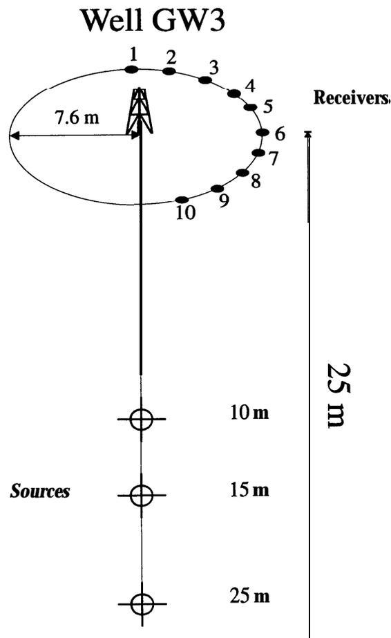
Figure 8. Schematic illustration of the acquisition geometry used for the azimuthal RVSP showing the Conoco rotary source and three-component surface geophone positions, shown as crossed circles and filled circles, respectively.
