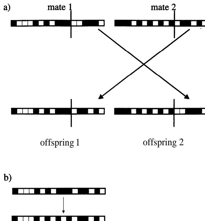
Figure 1. A schematic illustration of the operators employed by the genetic algorithm. The lines of black and white boxes represent a binary coding of a single model in the population. The crossover operator is illustrated in (a) where the two parent strings previously selected in the reproduction step exchange parts of their coding to produce two new offspring. In (b) the mutation operator is shown operating on a single bit in a models binary representation selected at random.
