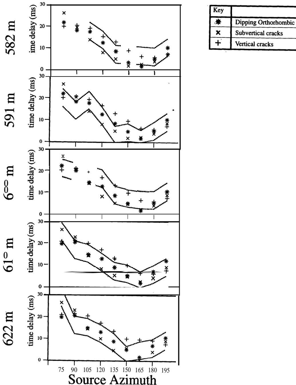
Figure 6. Time-delays between the fast and slow split shear waves corresponding to the optimal models found by the GA for different parametrizations. The dashed lines indicate the upper and lower estimated error bounds for the observed time-delays. Breaks in the dashed lines indicate that no data was available.
