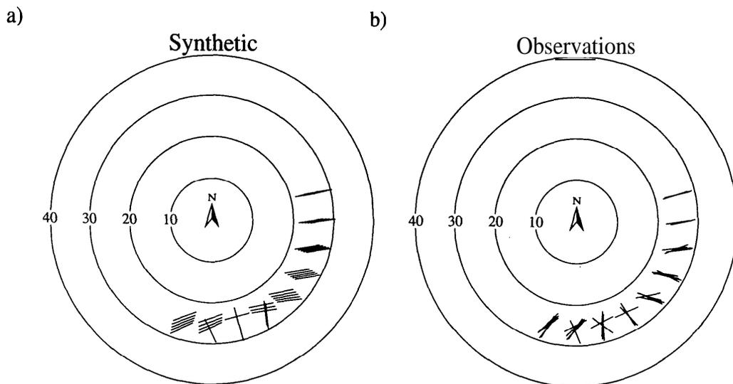
Figure 10. Polarization of the  $qS1$  shear waves measured from north for (a) the synthetic model observations and (b) the field observations plotted on a lower hemisphere equal area plot.
