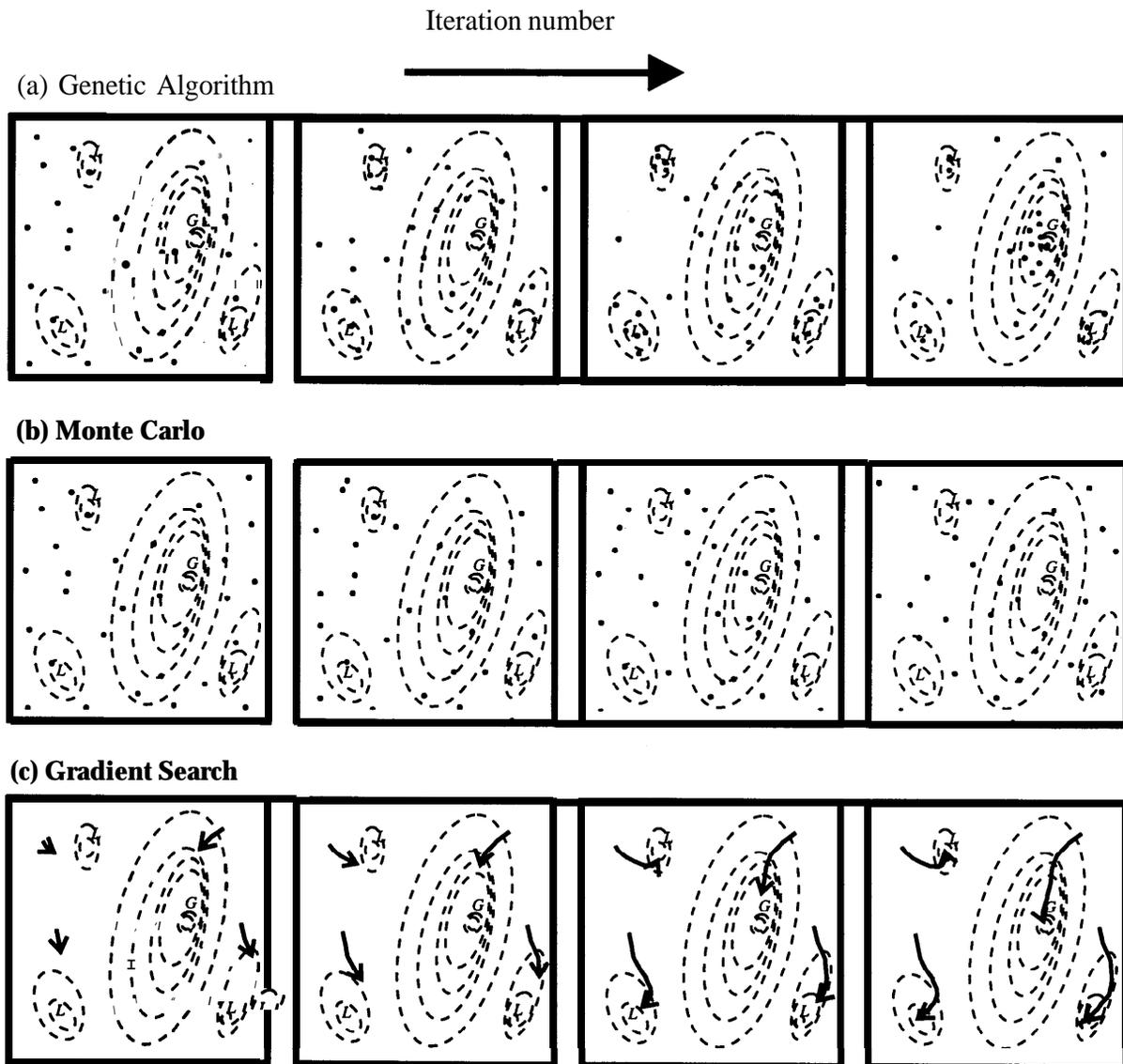
Figure 2. Schematic illustration of (a) a GA, (b) simple Monte Carlo and (c) local gradient searches for the optimization of a multimodal function in two dimensions during the iteration of the various methods. The Ls denote local optima and Gs the global optimum. For (a) and (b) the black dots indicate solutions sampled by the algorithms and for (c) the arrowed paths indicate the search directions from various starting models.
