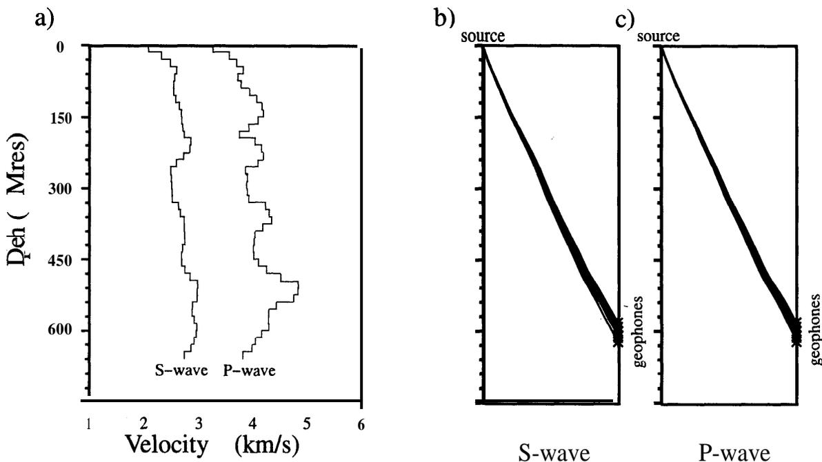
Figure 4. The velocity structure at the CBTF for both P- and S-waves as derived from sonic logs obtained in well 33-1. Isotropic ray tracing for both P- and shear-waves are shown in (b) and (c) for source and geophone positions corresponding to the azimuthal VSP geometry.
