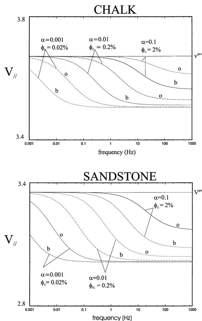
FIG. 3. Velocity dispersion corresponding to Figure 2, for oil-filled (o) and brine-filled (b) cracks, and different aspect ratios  $\alpha$ . Oil moves the curves to lower frequencies, so too does a reduction in aspect ratio.  $V^{gas}$  is the velocity for completely gas-saturated cracks.
