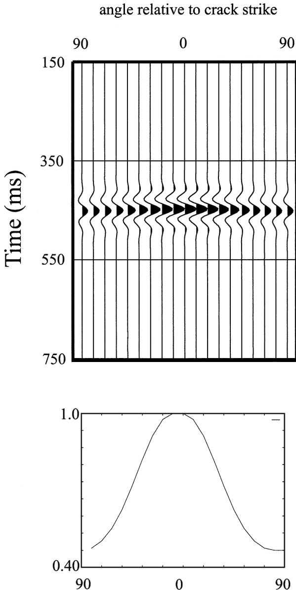
FIG. 5. Synthetic seismogram showing a common receiver gather at 1400 m from an azimuthal VSP with an offset of 700 m. The peak frequency of the wavelet is 30 Hz. Note the strong decrease in amplitude perpendicular to the crack strike. The material is an anisotropic sandstone, the cracks saturated with brine, and the matrix properties given by Table 1. There is a velocity anisotropy of 5%. The lower diagram shows the average amplitude.
