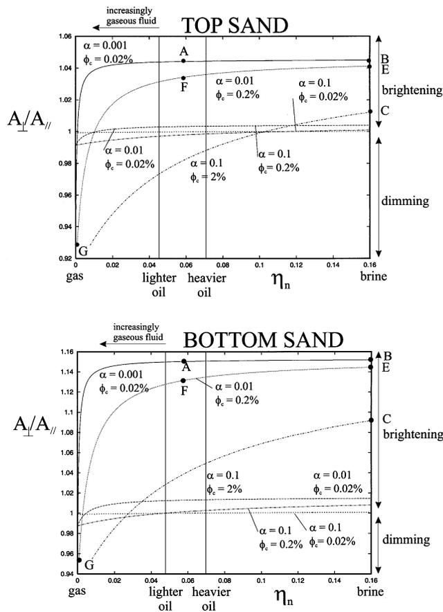
FIG. 7. Ratio of reflected amplitudes perpendicular and parallel to the crack strike for continuous fill variation ( $\eta_n = \rho_{liq} V_{liq}^2 / \rho V_p^2$ ) different aspect ratios ( $\alpha$ ), and porosities  $\phi_c$ . Solid circles correspond to points in this plot chosen for later synthetic seismogram modeling.
