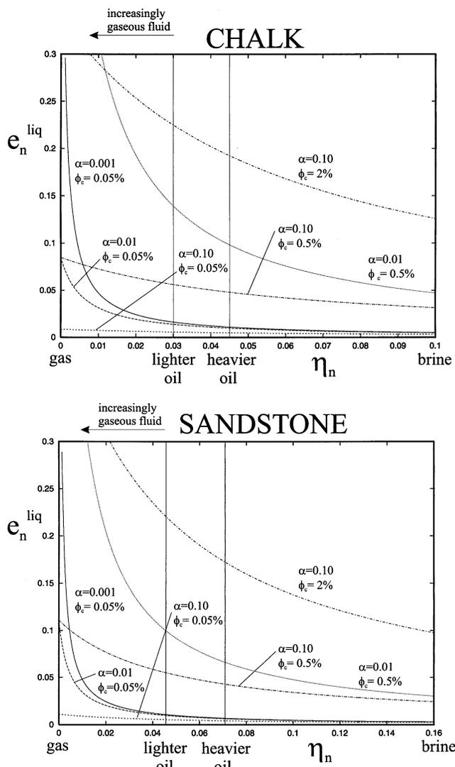
FIG. 1. Variation in crack stiffness for continuously changing fill parameter  $\eta_n$  ( $=\rho_{liq}/V_{liq}^2/\rho V_p^2$ ) and different aspect ratios ( $\alpha$ ). The vertical lines demarcate conditions appropriate to most produced hydrocarbons according to Batzle and Wang (1992). The other crack index,  $e_r^{liq}$ , is invariant with fill. Different crack porosities,  $\phi_c$ , are considered, with the largest being the upper limit using the theory in this paper.
