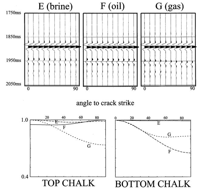
FIG. 10. Synthetic seismograms for a chalk reservoir with cracks possessing an aspect ratio of 0.01 and brine (E), oil (F), and gas (G) fills. The crack conditions correspond to points E, F, and G in Figures 4 and 6. Averaged amplitudes are shown for each event.
