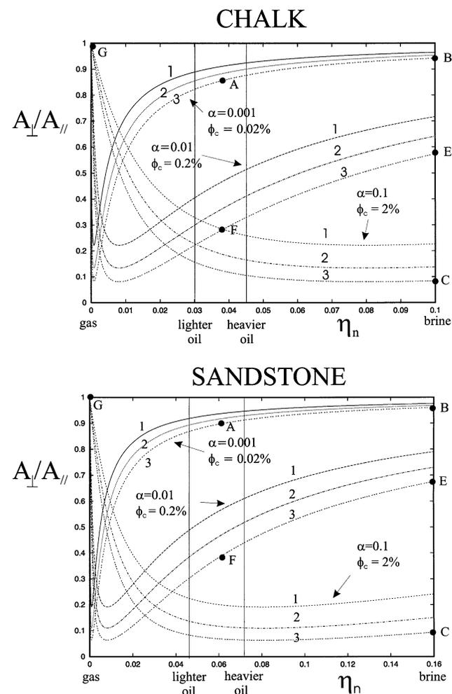
FIG. 4. Ratio of amplitudes perpendicular and parallel to the crack strike for horizontal wave propagation and the attenuation mechanism proposed in equation (14). Calculations are for a frequency of 30 Hz and range of fluid fills defined by the parameter  $\eta_n (= \rho_{liq} V_{liq}^2 / \rho V_p^2)$ . Numbers indicate pathlengths: 1—300 m, 2—400 m, 3—500 m. Labeled filled circles correspond to points in this plot chosen for later synthetic seismogram modeling.
