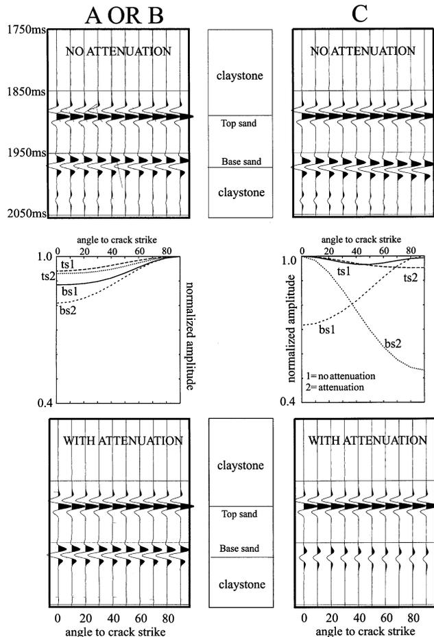
FIG. 9. Synthetic seismograms for a 150-m-thick sandstone reservoir. Averaged amplitudes for each event are shown in the central diagram, and the top (ts) and base (bs) events, with (bottom) and without (top) attenuation. Calculations are for brine- and oil-filled cracks with an aspect ratio of 0.001 (A or B) and brine-filled cracks with an aspect ratio of 0.1 (C). Labels correspond to points in Figures 4 and 7. Seismograms are normalized by the maximum amplitude for the top event.
