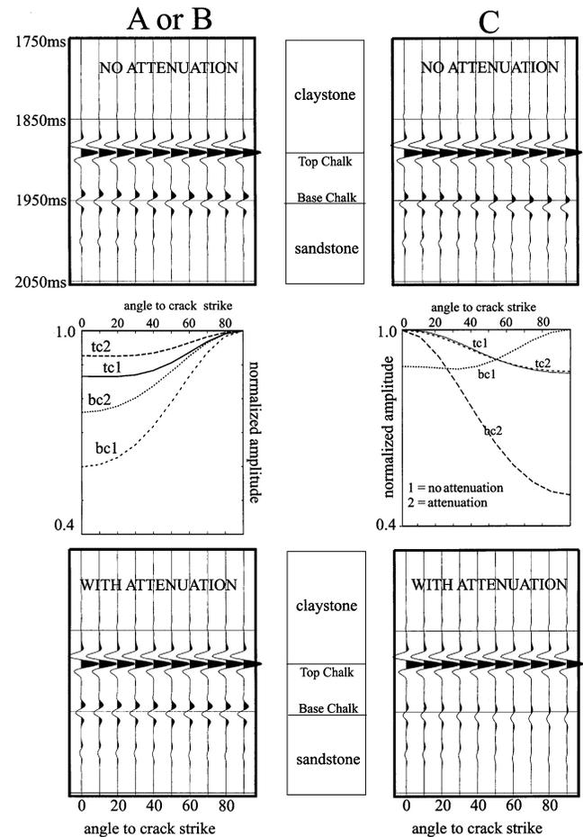
FIG. 8. Synthetic seismograms for a 150-m-thick chalk reservoir, with (bottom) and without (top) crack-related attenuation. Averaged amplitudes for each event are shown in the central diagram, with the top (tc) and base (bc) events. The cracks are brine or oil filled (A or B) with an aspect ratio of 0.001, or brine filled with an aspect ratio of 0.1 (C). The labels correspond to the points in Figures 4 and 6. Seismograms are normalized with respect to the largest amplitude for the top event.
