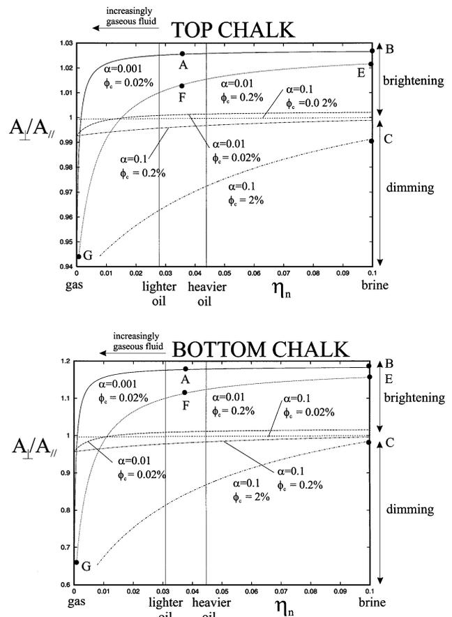
FIG. 6. Ratio of reflected amplitudes perpendicular and parallel to the crack strike for continuous fill variation ( $\eta_n = \rho_{liq} V_{liq}^2 / \rho V_p^2$ ), and different aspect ratios ( $\alpha$ ) and porosities. Solid circles correspond to points in this plot chosen for later synthetic seismogram modeling.
