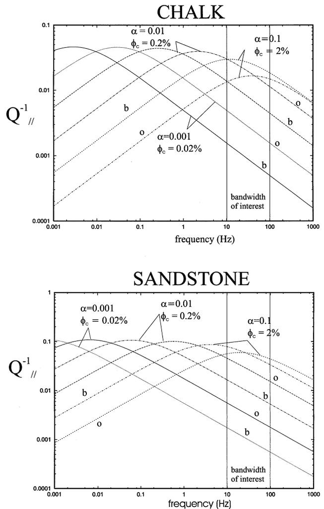
FIG. 2. Dimensionless  $Q_{//}^{-1}$  factor for horizontal propagation parallel to the crack strike. Curves are for oil (o) and brine (b) fill, and also different aspect ratios  $\alpha$ . Brine moves the peaks to lower frequencies, so too does a reduction in aspect ratio. Curves are based on the attenuation law defined in equation (14), with a characteristic time constant of 40 ms.
