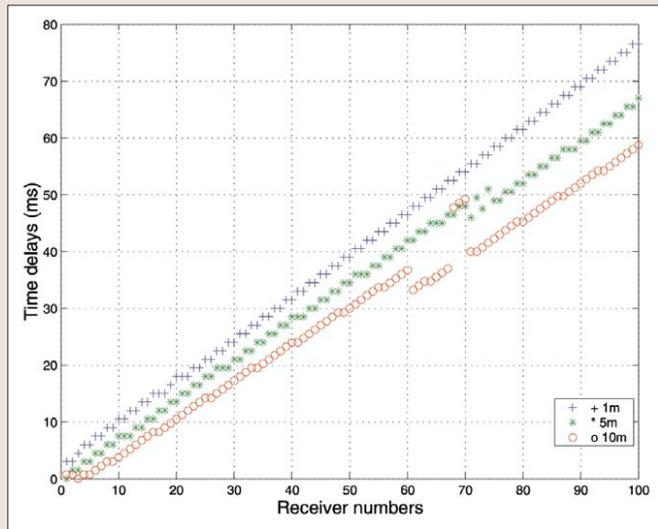
Figure 4. Variations of time-delays of split shear-waves with receiver numbers (depth) computed from synthetic four-component data for three different fracture sizes.
