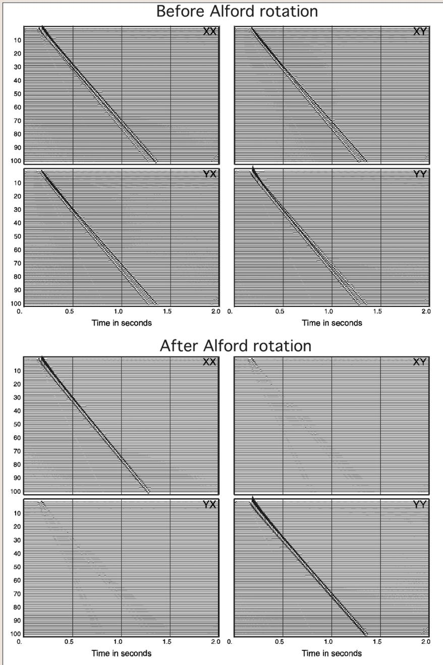
Figure 2. Synthetic four-component shear-wave data (top) that have been rotated to the natural coordinates (bottom).
