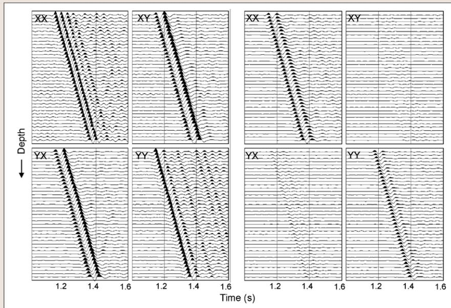
Figure 5. Bluebell-Altamont four-component shear-wave data (left) that have been rotated to the natural coordinates (right).
