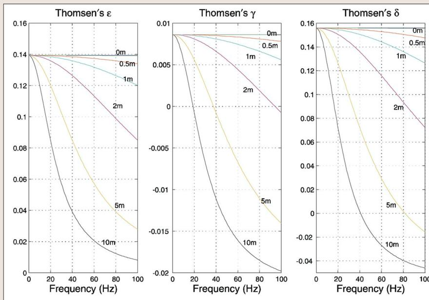
Figure 1. Variation of Thomsen's three anisotropic parameters with frequency computed for different fracture sizes (see text for parameters used).
