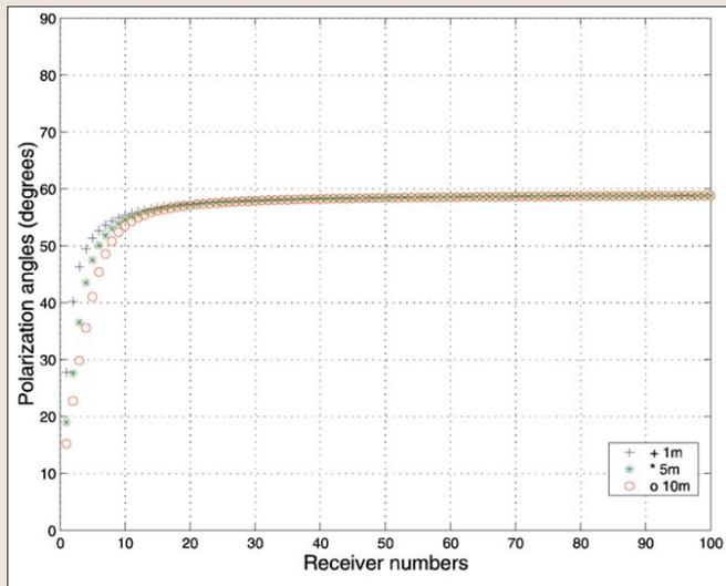
Figure 3. Variations of polarizations of fast split shear-waves with receiver numbers (depth) computed from synthetic four-component data for three different fracture sizes. The angles are relative to the in-line component.
