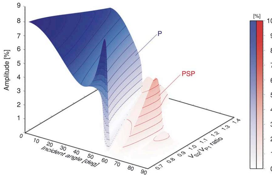
Figure 6 Effective reflection coefficients for the pure P-wave and the PSP-mode as a function of incident angle and a varying ratio of the S-wave velocity of the basalt ( $V_{S2}$ ) to P-wave velocities of the overlying and underlying rocks ( $V_{P1}$ ).
