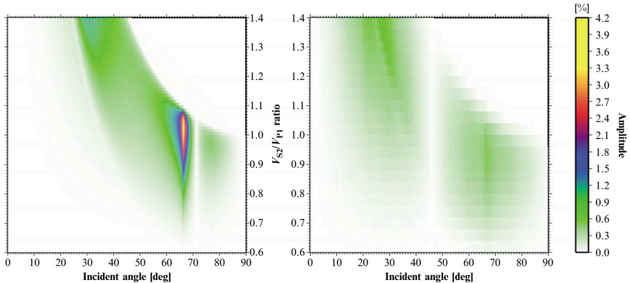
**Figure 5** Effective reflection coefficients as a function of incident angle and a varying ratio of the S-wave velocity of the basalt ( $V_{S2}$ ) to P-wave velocities of the overlying and underlying rocks ( $V_{P1}$ ). Left: for the PSP-mode; right: for the PSS-mode.
