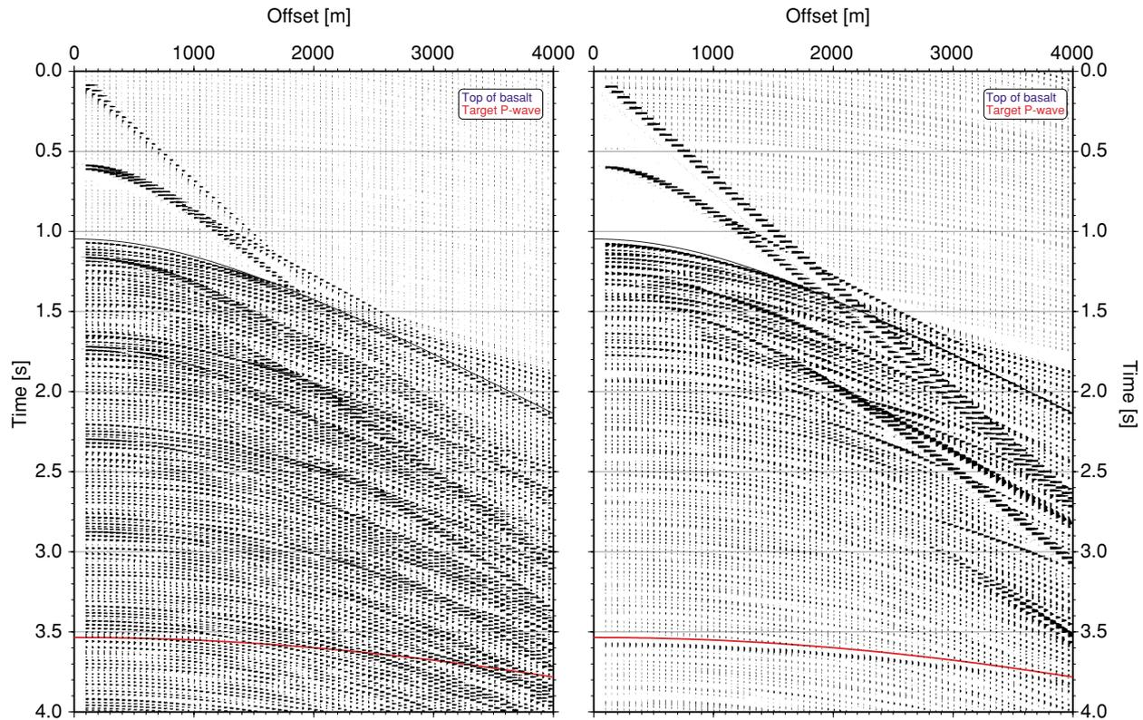
**Figure 9** Synthetic seismograms for the multilayered basalt model of Fig. 8, showing P-wave traveltim curves for reflections from the top of the basalt (blue) and the sub-basalt interface (red). Left: including sea-surface; right: without sea-surface.
