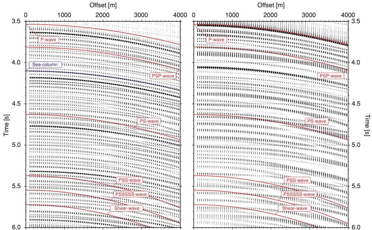
Figure 10 Shot gathers showing the seismic response of the sub-basalt interface only (see text for details) with plotted traveltime curves for associated target reflections. Left: including sea-surface; right: without sea-surface.
