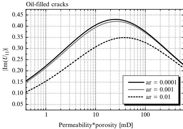
**Figure 13** As Fig. 12 for oil-filled cracks (increased viscosity, see Table 3). The maximum is moved to higher permeability and porosity values.
