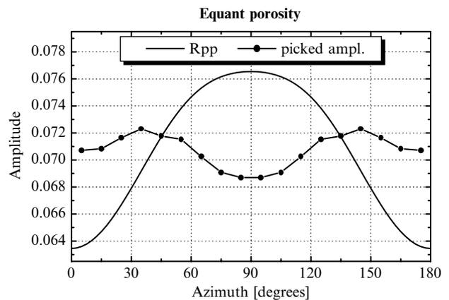
**Figure 15** Synthetic data example from Fig. 6 with attenuation due to equant porosity in the fractured layer. The porosity is 10% and the permeability 50 mD. The azimuthal amplitude variation that the reflectivity produces (solid line) is cancelled in the data (points) by attenuation. Even the symmetry orientations will not be detectable.
