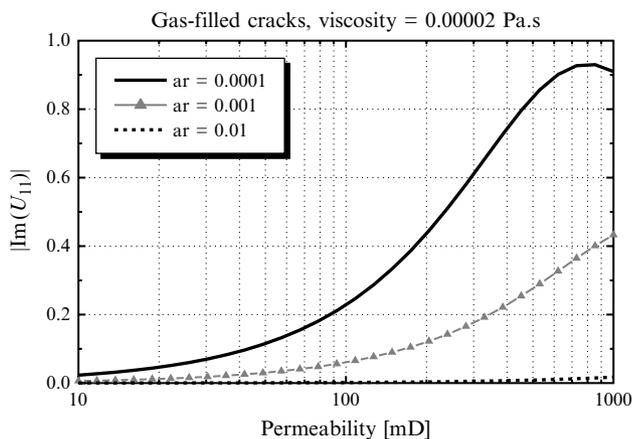
**Figure 9** As Fig. 8 for a model with gas-filled cracks. Values are increased (compare vertical scales of Figs 8 and 9) and a maximum is reached at an aspect ratio of 0.0001 and high permeabilities.
