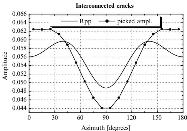
**Figure 11** Synthetic data example, showing the effect of attenuation due to interconnected cracks on the amplitudes. The model contains gas-filled cracks with an aspect ratio of  $10^{-4}$ , a crack density of 0.1, and the permeability is 1D. Points are amplitudes picked from the data and the solid line shows the reflection coefficient for comparison. The symmetry directions are still detectable, but the estimation of correct crack parameters will not be possible.
