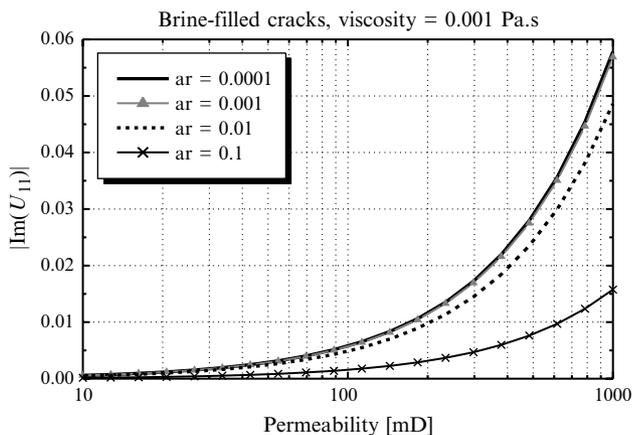
**Figure 8** Dependence of the imaginary part of  $U_{11}$  on permeability and aspect ratio for interconnected cracks at a frequency of 30 Hz. Cracks are brine-filled. Values increase with permeability and decrease with aspect ratio.
