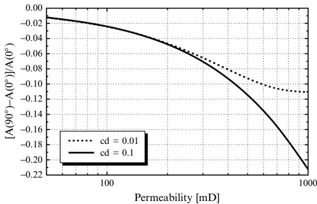
**Figure 10** Interconnected cracks, relative change in attenuated amplitudes between the symmetry directions,  $[A(90^\circ) - A(0^\circ)]/A(0^\circ)$ , for gas fill and an aspect ratio of  $10^{-4}$ . Variation with permeability and crack density. Amplitudes were computed at an incident phase angle of  $40^\circ$ . The azimuthal amplitude variation is significant for permeabilities from 500 mD to 1 D and it increases strongly with crack density over that range.
