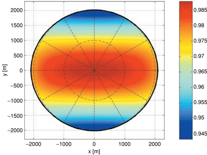
**Figure 7** Transmission coefficients at the top of the HTI layer for a model with brine-filled cracks, a crack density of 0.1 and an aspect ratio of 0.001. The azimuthal variation is very small and maximum amplitude changes between the symmetry directions are 2%. (An offset of 2000 m corresponds to an angle of incidence of approximately 43°.)
