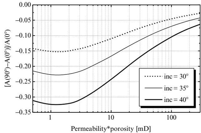
**Figure 14** Relative change in amplitudes between the fracture strike and the fracture normal due to attenuation for equant porosity. Dependence on *permeability\*porosity*. Cracks are brine-filled with an aspect ratio of 0.001 and a crack density of 0.1. Values are evaluated at incident phase angles of 30°, 35° and 40°. They exceed 10% for almost the entire range of permeability and porosity values.
