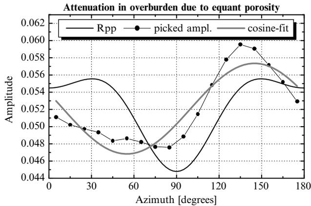
**Figure 17** Attenuation in a fractured overburden with a fracture strike different from that of the target layer (see Table 4 for the model parameters). The signature of the reflection coefficient (black solid line) is altered completely. The amplitude data (dots), picked at an angle of incidence of  $41^\circ$ , suggest incorrect orientations of the symmetry planes shown by the grey solid line.
