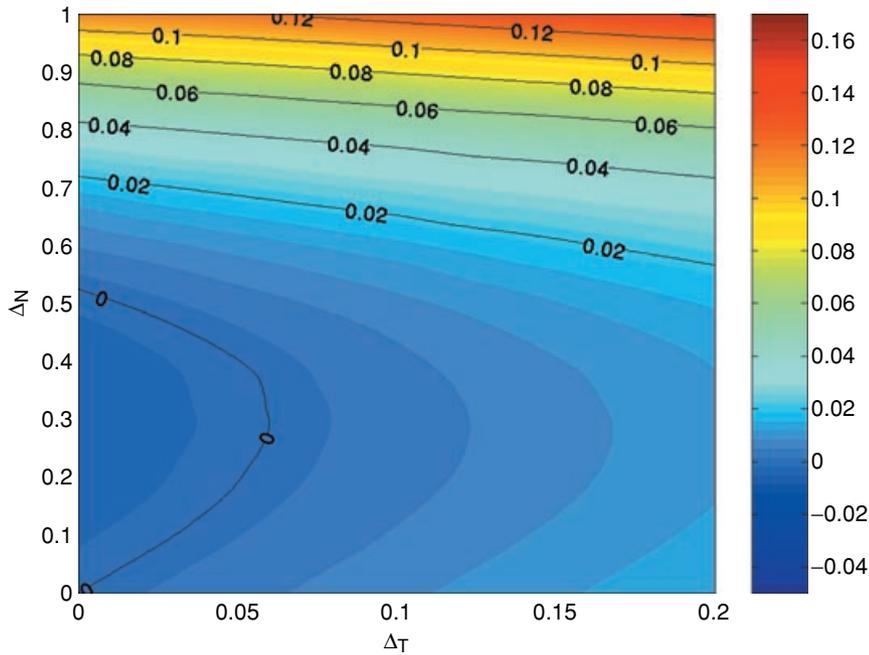
Figure 4 Relative change in divergence factors between the symmetry directions for  $v_s/v_p=0.35$  and a layer thickness of 300 m at an incident phase angle of  $30^\circ$ . The maximum values occur for high  $\Delta_N$  and increase with  $\Delta_T$  (=gas-filled cracks with a high crack porosity).
