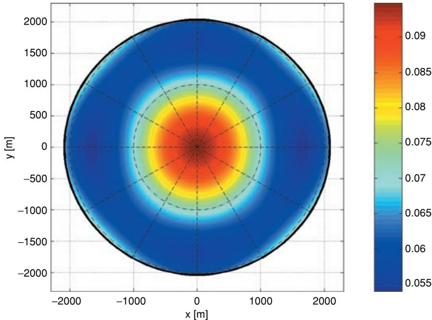
**Figure 16** Reflected and attenuated amplitudes for the model used in Figs 1, 6 and 15. The two effects cancel each other out at all offsets, so that the resulting amplitude signature does not vary with azimuth. The amplitudes give no indication of fracturing in the target, unless the effect of attenuation is removed.
