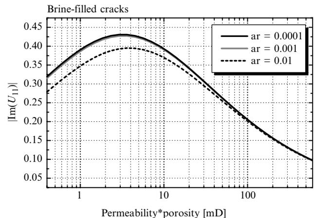
**Figure 12** Equant porosity; dependence of the imaginary part of  $U_{11}$  on *permeability\*porosity* for different aspect ratios. Cracks are brine-filled (see Table 3 for fluid properties). Maximum values lie at the lower end of the *permeability\*porosity* scale.
